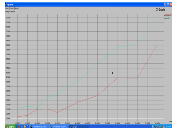
Fig 4.2.2: Routing overhead vs number of nodes
