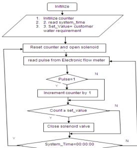
Fig. 5: Software flowchart for closed loop water metering
