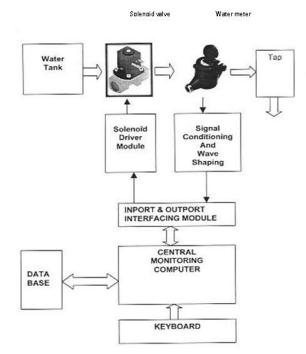
Fig. 2a: Single Channel Water Metering System
