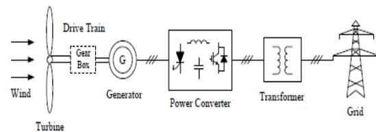
**Figure 1: Basic components of wind energy conversion system**
