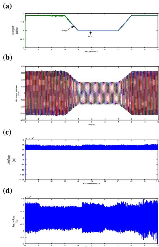
**Figure 9: Power flow response in wind speed step changes (from 12 to 10 m/s at 3 s and from 10 to 12 m/s at 7s). (a) Generator speed. (b) Generator output voltage (c) Grid output real power. (d) Grid output reactive power.**
