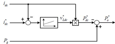
Figure 7: dc-link current regulator with generator power Feedforward [3].
