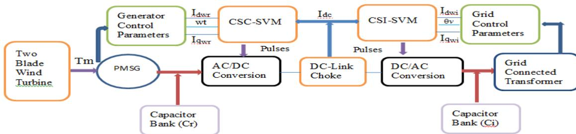
Figure 8: A wind energy conversion system using SVM-Technique
