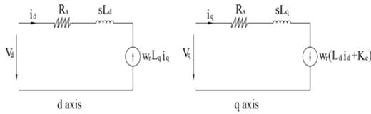
Figure 3: Equivalent circuit of PMSG in d-q reference frame
