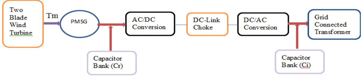
Figure 2: A wind energy conversion system using PWM CSR and PWM CSI.
