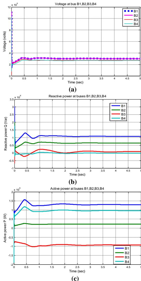
**Fig 5: Profiles at buses B1, B2, B3, B4 with STATCOM, (a) Voltage, (b) Active Power, (c) Reactive Power.**
