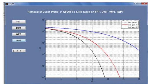
Figure 5. shows that performance comparison of SNR and bit error rate for WPT in SOFDM
