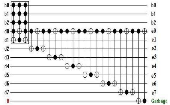
Figure 6: Circuit for Single bit left shifter
