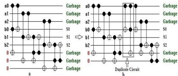
**Figure 7: Architecture for duplicate circuit**
