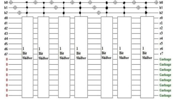
Figure 5: Circuit for 8bit left shifter
