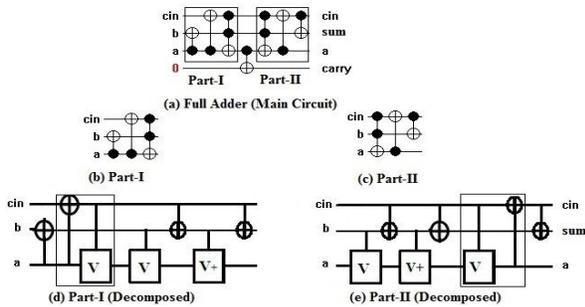
**Figure 9: Quantum Cost reduction for the Adder with optimal garbage**
