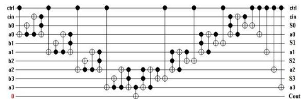
**Figure 4: Optimized Adder/Subtractor Circuit using only one constant input**
