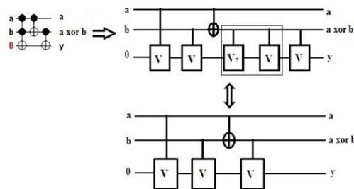
**Figure 8: Quantum Cost reduction for XOR-OR Circuit**
