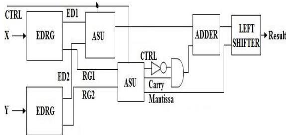
**Figure 2: Schematic Diagram for Logarithmic Multiplier and Divider**
