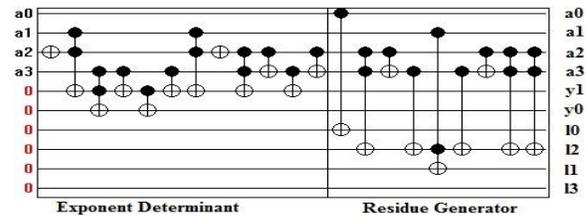
**Figure 3: Architecture for Four bit Exponent Determinant and Residue Generator**
