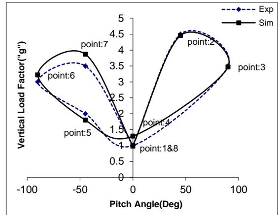
**Figure 5: Comparing vertical charge factors of simulation and on experimental basis in different pitch angles during performance of Loop Maneuver**
