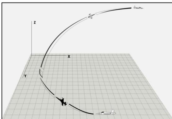
**Figure 3: Performance Schematic Figure of Chandelle Maneuver**
