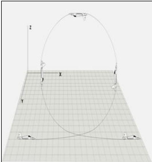
**Figure 2: Performance method of Loop Maneuver**
