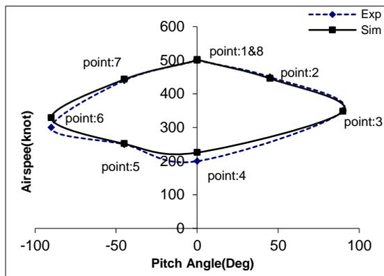
**Figure 4: Comparing airspeeds of simulation and on experimental basis in different pitch angles during performance of Loop Maneuver**
