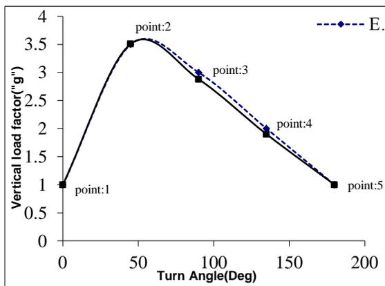
**Figure 7: Comparing vertical load factors obtained from flight simulation and on experimental basis in different turn angles during performance of Chandelle Maneuver**
