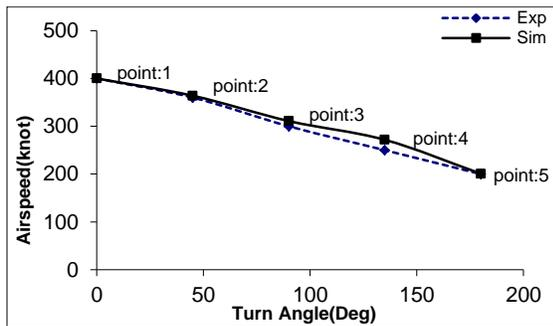
**Figure 6: Comparing airspeeds obtained from flight simulation and on experimental basis in different positions of turn angles during performance of Chandelle Maneuver**
