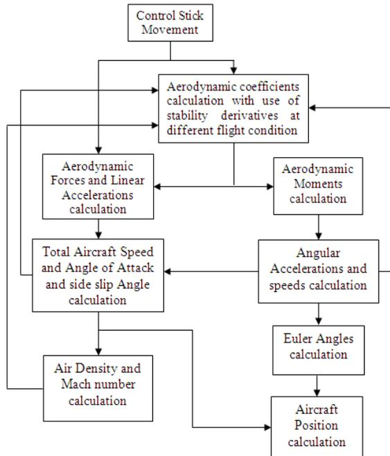
**Figure 1: Functional Scheme of flight Simulation**
