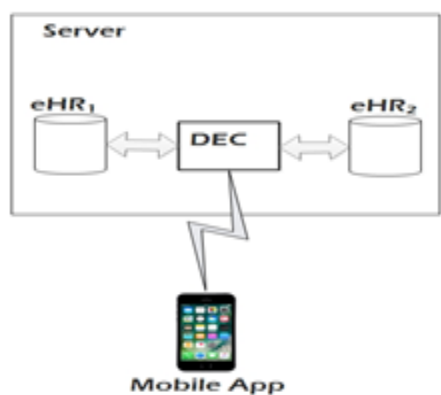
Figure 3 Setup IIIA-single server; physical/local server host setup
