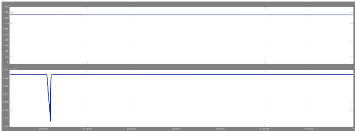
Fig 10: output waveform across the R-load and duty cycle of type-3 compensator
