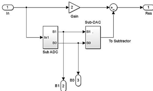
**Figure 7. MATLAB circuit diagram of a stage**
