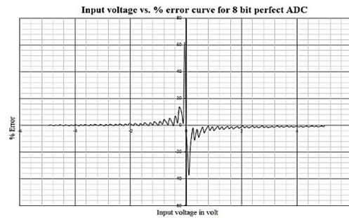
**Figure 12a:  $V_{in}$  vs.  $E_1$  graph**
