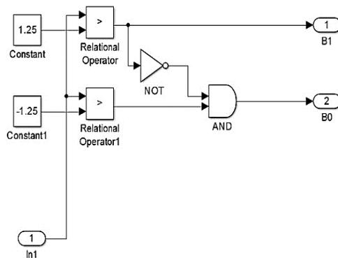
**Figure 8. MATLAB circuit of SADC**
