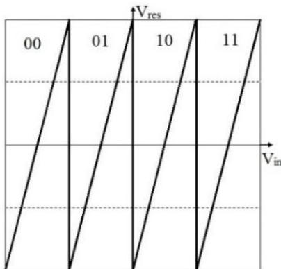
**Figure 1. Transfer curve of a 2 bit ADC**
