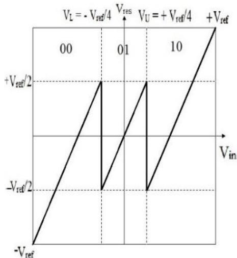
**Figure 4. Transfer curve for 1.5 bits/stage**
