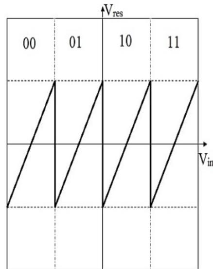
**Figure 3. Transfer curve with reduced gain**
