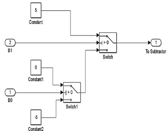
**Figure 9. MATLAB circuit of SDAC**
