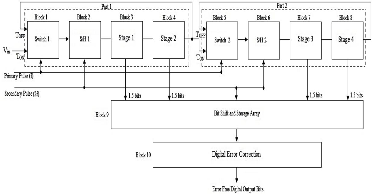
Figure 5. Block diagram of the proposed circuit
