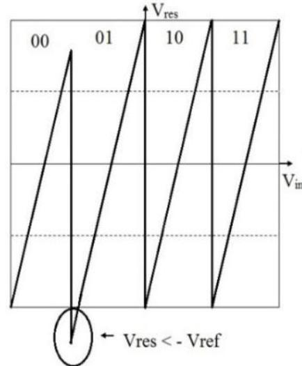
**Figure 2. Out of range error**
