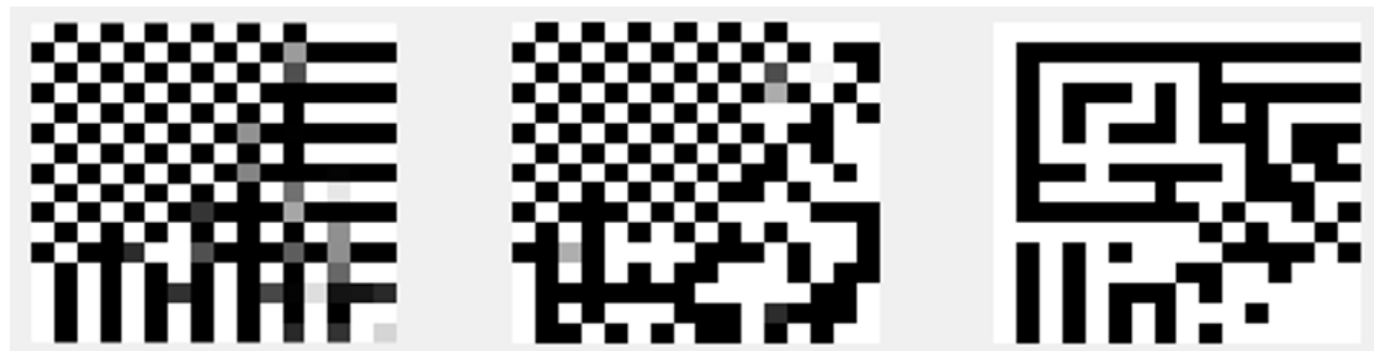
Figure 8 16X16 DCT of the images from left to right; grayscale image, anisotropic filtered image, anisotropic in addition to Laplacian-Gaussian filtered image
