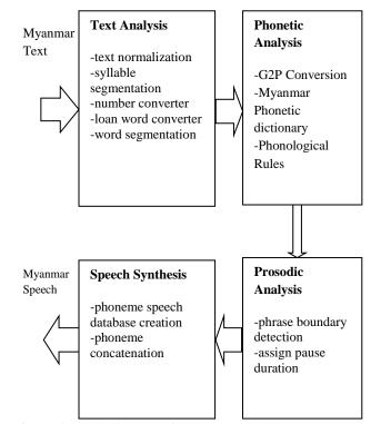
Figure 1 Block diagram of phoneme based Myanmar TTS system
