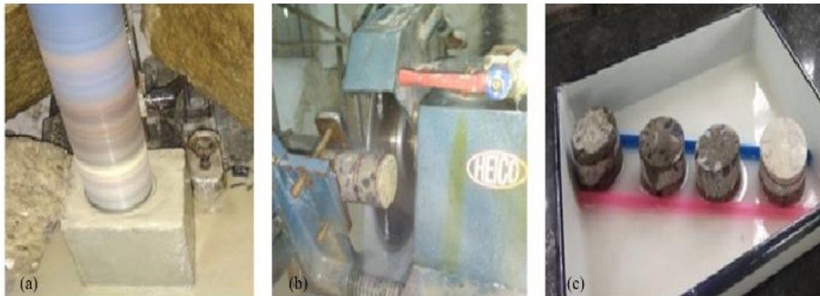
Figure 11 Sorptivity test setup (a) core cutting, (b) sample preparation, and (c) sorptivity test
