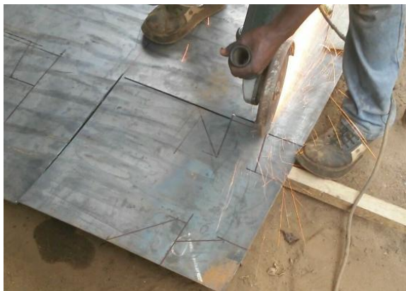
Figure 11 Marking and cutting out of the soybean thresher components
