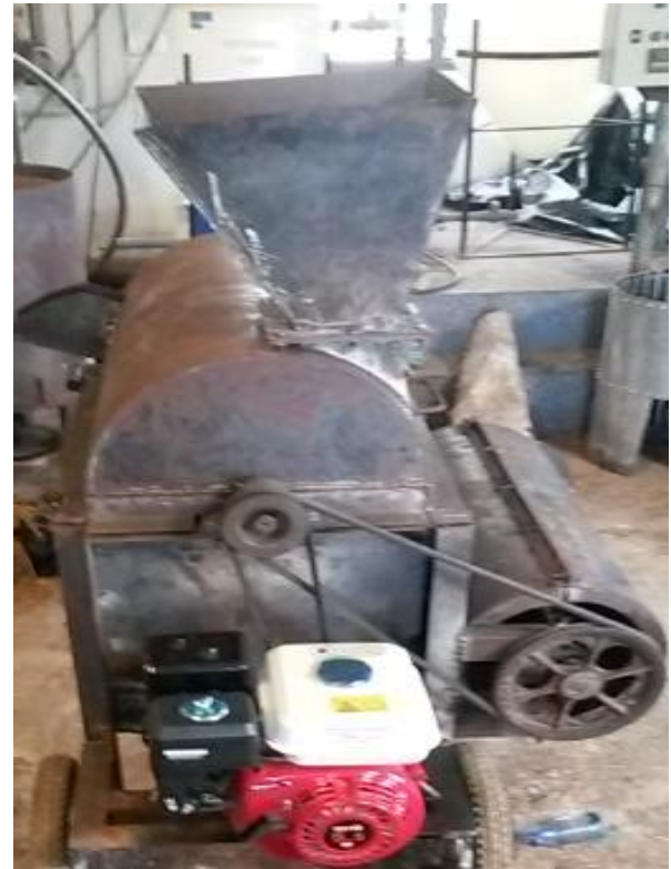
Figure 15 Photograph of the mechanical soybean thresher
