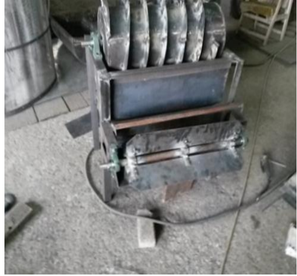
Figure 14 Fabricated components (threshing and cleaning unit) of the mechanical soybean thresher
