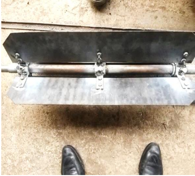
Figure 13 Fabricated component (blower/fan) of the mechanical soybean thresher
