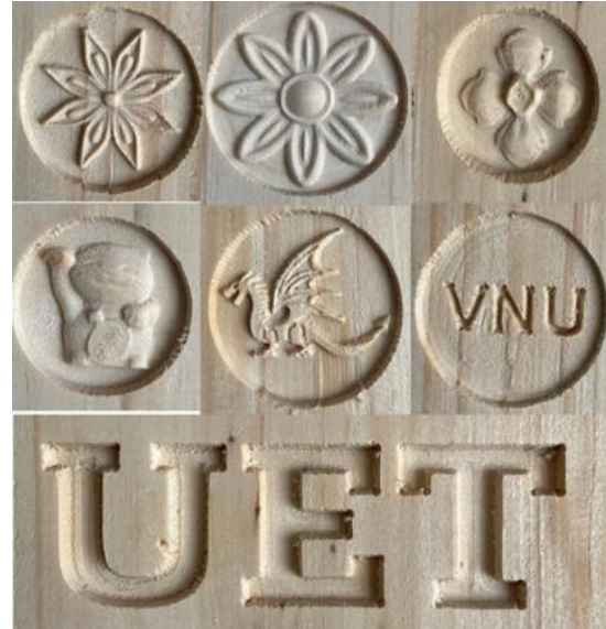
Figure 10 Sample engraved products created using the 3-axis CNC wood engraving machine
