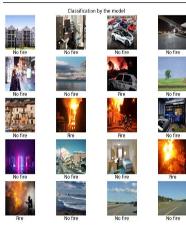
Figure 9 Fire and non-fire image classification using the VGG-16 model
