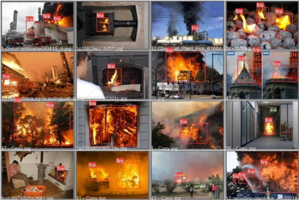
Figure 13 Validation batches detected by the trained YOLOv5 model
