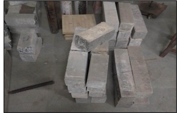
Figure 7 Fractured rectangular beam specimen
