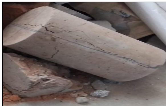
Figure 6 Fractured cube and cylinder sample
