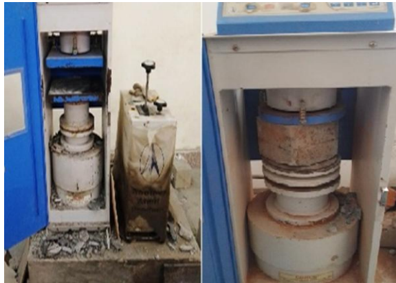
Figure 5 Digital compression testing machine
