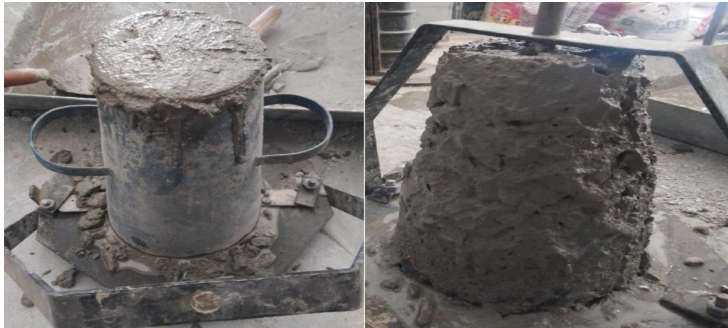
Figure 3 Slump cone test
