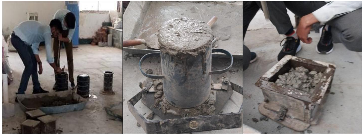
Figure 2 Mixing and casting of concrete
