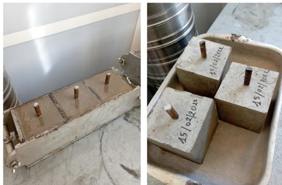
Figure 3 The reinforced concrete specimens used
