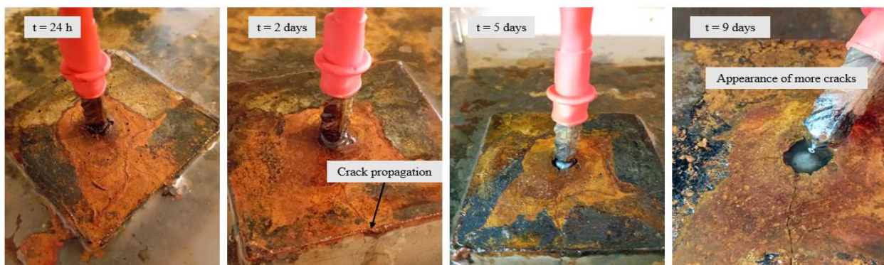
Figure 10 Crack development on specimen 3
