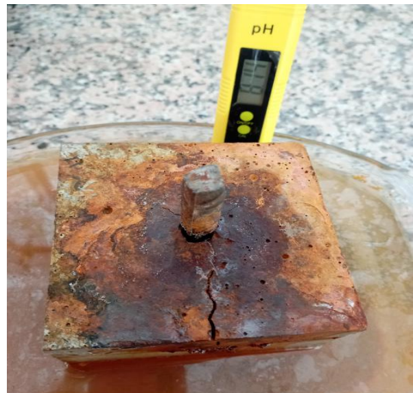
Figure 7 pH measurement after the corrosion test
