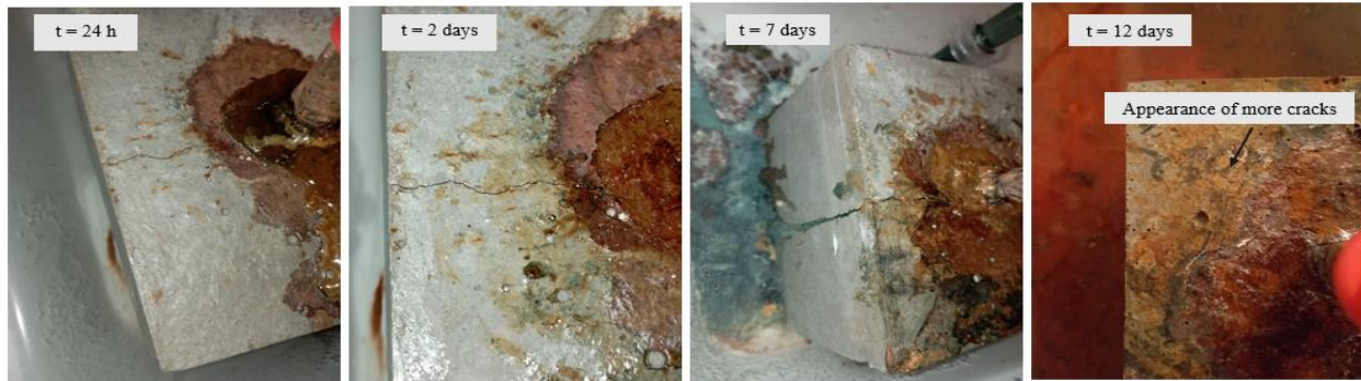
Figure 8 Crack development on specimen 1
