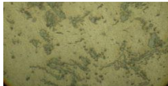
Figure 4 (c) Optical image of Al-15% FA composite
