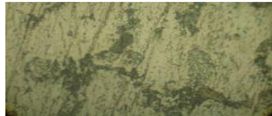
Figure 4 (b) Optical micrograph of Al-10% FA composite
