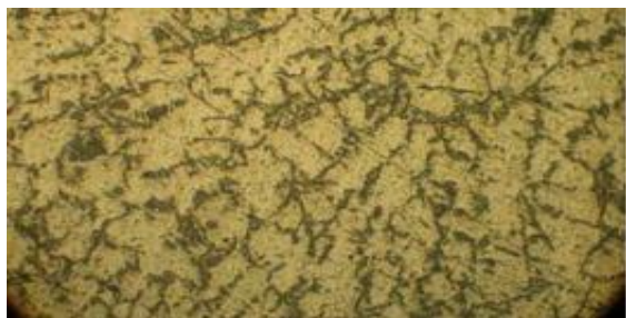
Figure 4 (e) Optical micrograph of the Al-2% Si-10% FA composite
