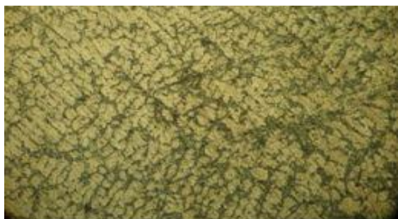
Figure 4 (f) Optical micrograph of the Al-2% Mg-10% FA composite
