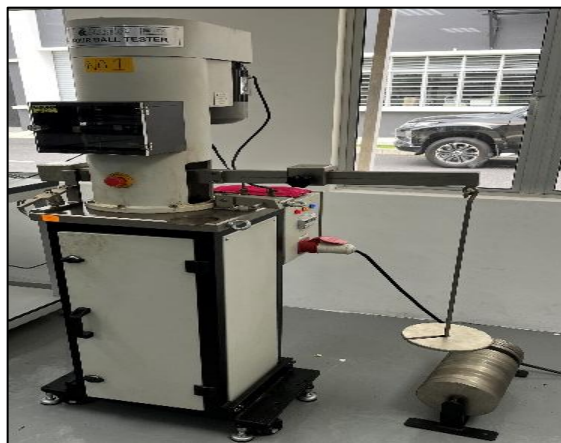
Figure 5 Koehler model K93190-M-CE 4-ball testing
