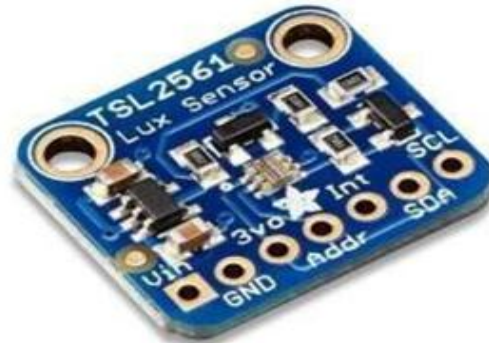
Figure 6 TSL2561 digital luminosity sensor [11]
